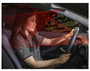
resume driving in manual mode, in Level 3 and 4 automated vehicles. And in "manually driven" cars, the Valeo Driver Monitoring System technology can help reduce accidents related to fatigue and distraction (these account for 54% of fatal accidents in Europe).
