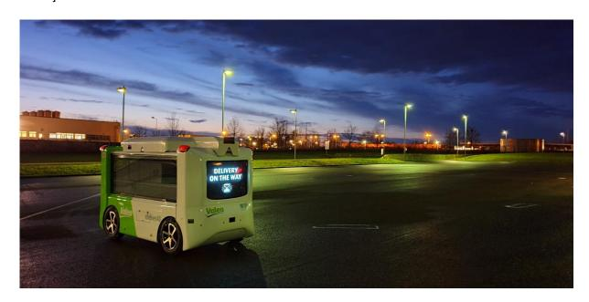
Finally, Valeo eDeliver4U brings together plug & play visibility, lighting and signaling systems that are immediately ready to use. The goal is multifaceted: keep sensors operational no matter the conditions [see technical details below]; let the droid see and be seen by everyone, especially pedestrians; and communicate using HD-resolution screens, with people interacting with the droid.
