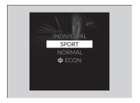
Enhances heightened throttle and steering response and modified active sound control.
