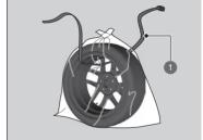
**4.** Bore through the bag, and pass the holding belt through the hole of the bag and the wheel of the flat tyre as shown.
