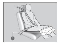
Deployed Passenger's Knee Airbag
