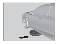
**6.** Place the compact spare tyre (wheel side up) under the vehicle body, near the tyre that needs to be replaced.
