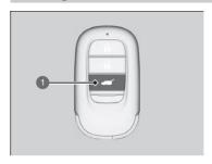
Press the hatch unlock button to unlock the hatch.
