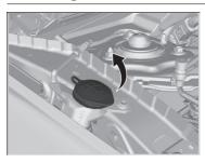
Open the cap and check the amount of window washer fluid.
