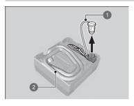
**1.** Take the air compressor hose and plug cord out of the back of the air compressor.
