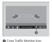
The system can be turned on and off on the audio/information screen by pressing the Cross Traffic Monitor icon.
