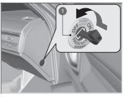
Passenger Front Airbag ON/ OFF Switch
