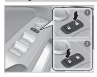
Press the master door lock switch in as shown to lock or unlock all the doors, hatch and fuel fill door.
