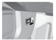
2 Locate the bonnet latch lever, push it to the side, and then raise the bonnet. Once you have raised the bonnet slightly, you can release the lever.
